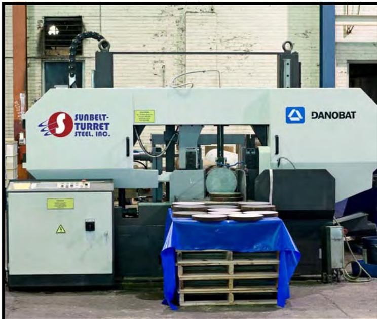
Charlotte was the lucky recipient of a new Danobat saw. This is the latest in cutting technology and has a cutting capacity of 20" diameter. Charlotte also has another new saw on order that will raise our cutting capacity to 32" diameters and should be in place in the coming weeks.
